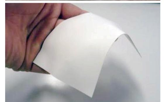
Gel sheet (t 0.3mm) containing 60vol% AlN (Not surface treated)
